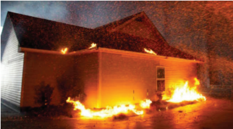
Figure 23: Richburg, S.C. - This ember storm simulation by the IIBH Research Center highlights common pathways of ignition. Photograph by The Insurance Institute for Business & Home Safety.
