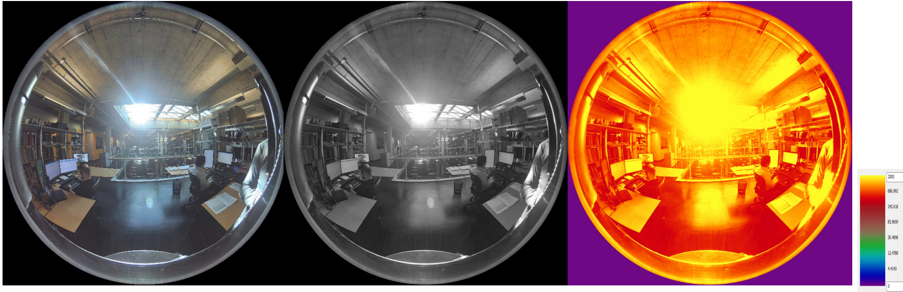
Workstation next to the skylight with direct sunlight DGP=0.375; Measured lux = 3700
