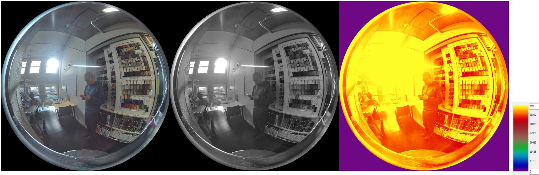
Library with reflected sunlight from the opposite building DGP=0.46; Measured lux = 5266
