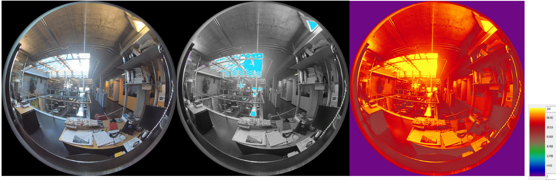
Workstation next to the skylight with diffused/reflected sunlight DGP=0.264; Measured lux = 1657
