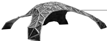
Degradation Movement (2016) Shell Mycelium / Kerala, India temporary pavilion for human shelter flexible wood structure; insulating layer produced by mycelium + soil substrate
