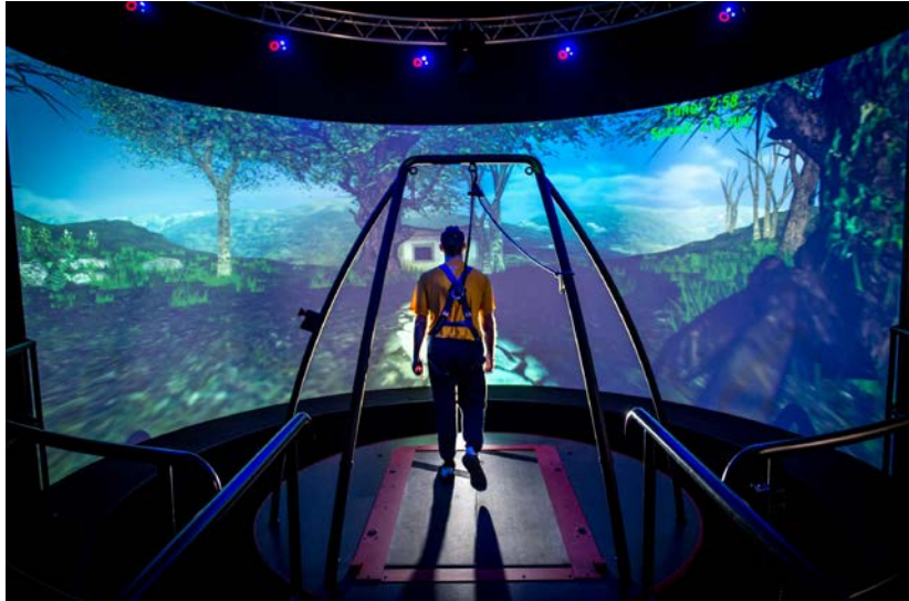
A traumatic brain injury patient walks through a virtual reality scenario at the Computer Assisted Rehabilitation Environment Laboratory at National Intrepid Center of Excellence at Walter Reed National Military Medical Center in Bethesda, Md., March 20, 2017. The patient is attached to a safety harness and walks on a treadmill on a platform that moves and rotates in conjunction with movements of the projected environment. Motion capture cameras track the patient's movements via reflective markers that are applied to the patient and supply data on physical deficits to physical therapists. Air Force photo by J.M. Eddins Jr. "The appearance of U.S. Department of Defense visual information does not imply or constitute DOD endorsement."
